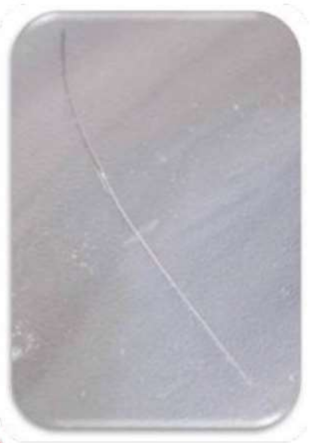
Cracks with heat damage (marks of overheating)
